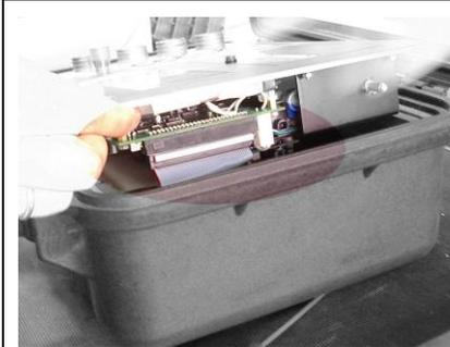
3. Undo the ribbon connection underneath the right edge of the front panel.
