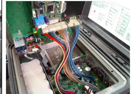
4. Turn the panel up over its right hand side and note the wire connections before undoing them.
