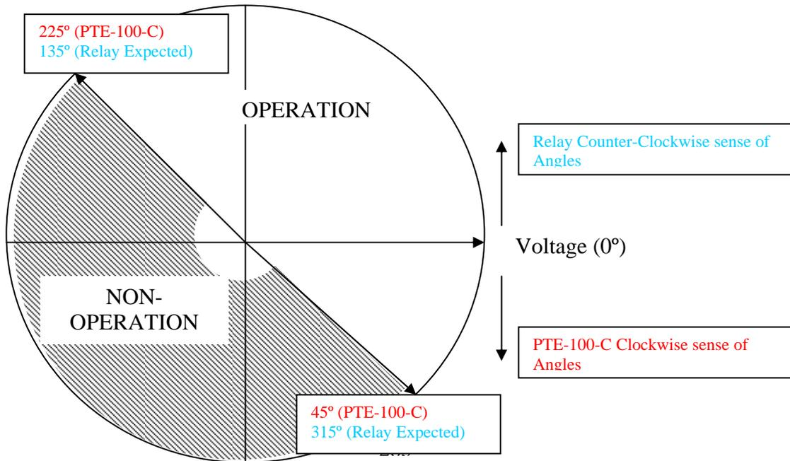
As a matter of fact, as it is evident in the figure, we are always able to apply when the Relay expected values (REV) and the Found Values by the PTE-100-C (FVPTE) the following formula to determine numerically the Operation Limits.
