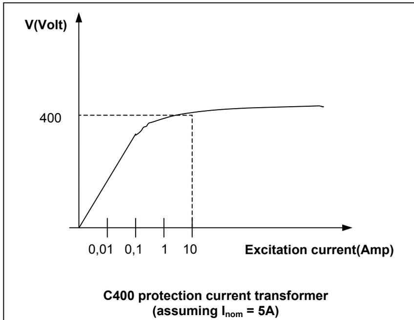
This concept is the one used for testing the knee-point in current transformers with the PTE-100-C.
