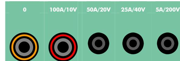
Tap zero is the common reference. If you are testing with currents ranging from 0 to 50 A AC, for example, connect the load between the common tap and the tap labeled "50 A / 20 V". If you are using 4 mm bananas, you will need the supplied 6-mm to 4-mm plug adapters for the common tap and the 100 A tap.
