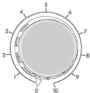
This knob controls the output level of the current and voltage power taps. The numerical 0-10 round scale is provided as a positional reference only. The actual output level is shown in Display #2 and, at any given regulator position, its value always depends on the connected impedance. Regardless of the regulator's position, no power will be output when the output control switch is OFF. Always handle this regulator with care.
