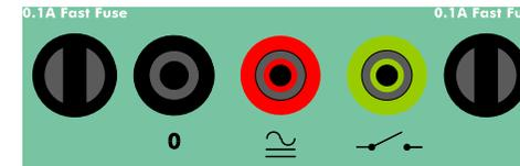
In its most typical implementation, a relay is said to *operate* when, upon detection of a fault, it closes its output contact to trip a circuit breaker, thus clearing the fault. The PTE-100-C will simulate the presence of a circuit breaker by means of its *trip monitor*, that will automatically stop both the timer *and* the power output when the relay operates, thus completing the *fault clearance* cycle.
