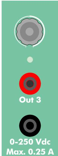
*Auxiliary Outputs* are intended as general purpose voltage supplies, rather than actual power sources. These outputs are also galvanically isolated from each other and from the main power supply.
