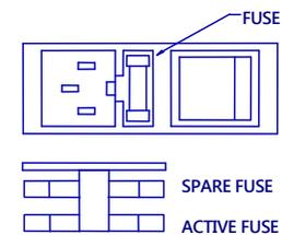
The active (12A, Fast) fuse and a spare fuse are included in the fuse holder. All the fuses accessible from the front panel are standard, 5x20 mm cylindrical, and their current rating and type are clearly printed.
