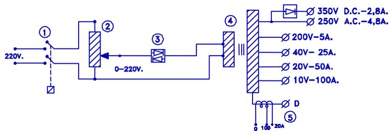
1. An internal relay connects the main power supply to the variac under no-load conditions.
