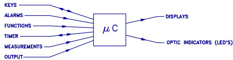
The same micro-controller processes all the user's control actions like output on/off, the timer activation, the selection and display of function values, and the protective alarms.
