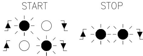
The timer will start when any PTE unit has transmitted a positive or negative signal, via the BUS-PTE and will stop when any PTE unit has transmitted specific signal, via the BUS-PTE.
