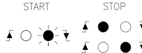
The timer will start when any PTE unit has transmitted a negative signal, via the BUS-PTE and will stop according to the signal programmed in M2
