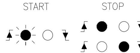
The timer will start when any PTE unit has transmitted a positive signal, via the BUS-PTE and will stop according to the signal programmed in M2.
