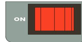
This is a normal, rocking switch located on the left-hand side of the front panel. The switch is indicated by the word ON. When the switch is ON, voltage is supplied to the unit.
