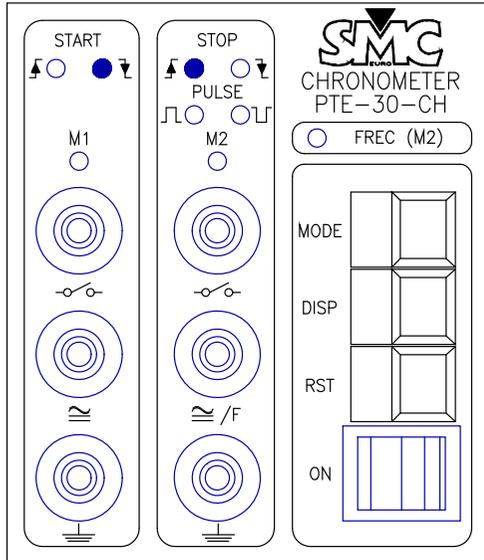
The timer will start when monitor M1 is deactivated and will stop when activated M2 is active. If the monitor M1 is not active when the timer is RESET, the timer will not start until the Monitor is active and is deactivated again.
