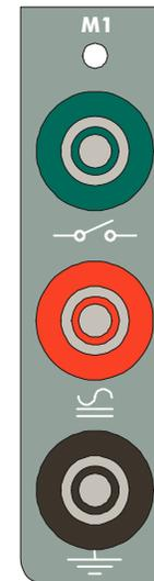
The monitor M1 has 3, 4mm taps, marked as follows. Common tap (black), power voltage input tap (red) and the dry contact or power free contract tap (green).
