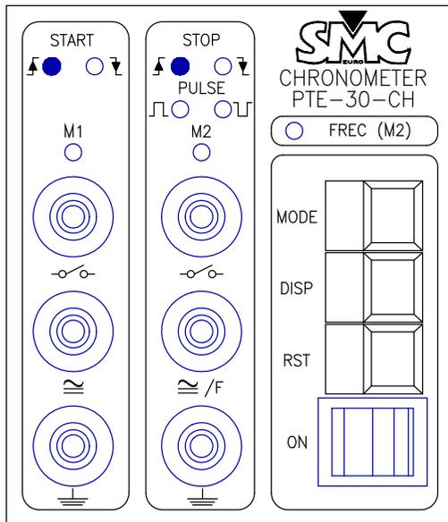
The timer will start when monitor M1 is activated and will stop when the monitor M2 is active. If the monitor M1 is active when the timer is RESET, the timer will not start until the Monitor is not active and is activated again.
