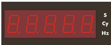
This highly efficient display consists of 5 digits of 7 segments, along with 3 luminous indicators, which show the reading, whether it be frequency, seconds, or cycles, automatically changing the decimal point.
