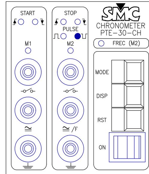
Timer starts when the monitor tap M2 is deactivated, and measures the time it is not active and stops when here is active.
