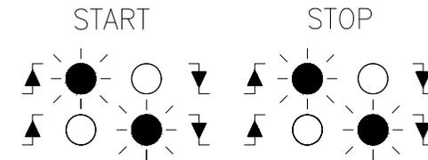
The timer will start when any PTE unit has transmitted a positive or negative signal, via the BUS-PTE and will stop when a negative or positive signal is transmitted
