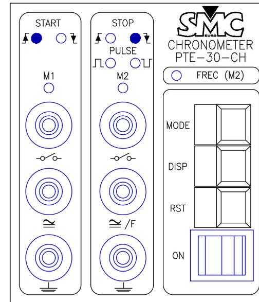
The timer will start when monitor M1 is activated and will stop when monitor M2 is not active. If the monitor M1 is active when the timer is RESET, the timer will not start until the Monitor is not active and is activated again.
