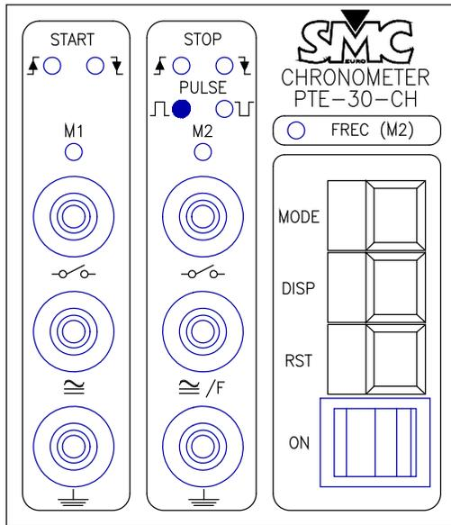
The timer starts when the taps M2 are activated, and measures the time of this active pulse. The timer will stop when it is deactivated.
