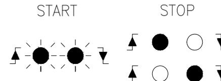
The timer will start when a PTE unit has transmitted via the BUS-PTE a specific signal and STOP according to what has been programmed in M2. The specific signal is made by software defined in the unit PTE and the specific signal is made by adequate test software.
