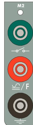
The monitor M2 has 3, 4mm taps, marked as follows. Common tap (black), power voltage input tap (red), and the dry contact or the power free contact tap (green).
