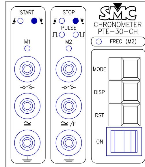
The timer will start when monitor M1 is deactivated and will stop when M2 is not active. If the monitor M1 is not active when the timer is RESET, the timer will not start until the Monitor is active and is deactivated again.
