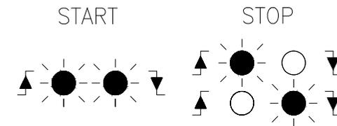
The timer will start when any PTE unit has transmitted specific signal, via the BUS-PTE and will stop when any PTE unit, via the BUS-PTE transmits a negative or positive signal.
