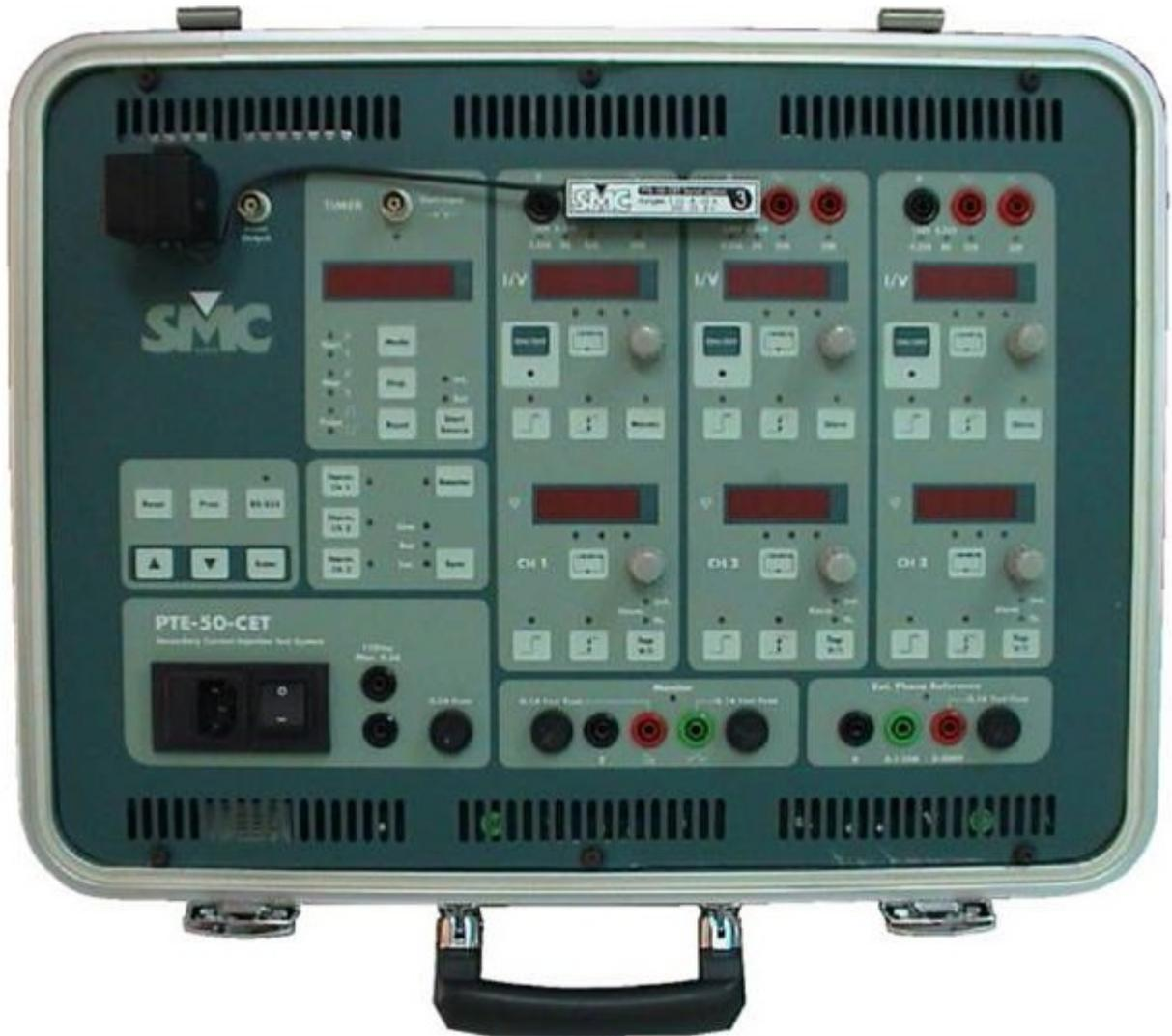
As seen in the picture the series bars connect to the PTE-50-CET only one way. Connections to the load are made on either side of the series bar. In the picture above the connection to the load would be made from the black common tap of channel one and the red polarity tap of channel two. Setting the current amplitude and phase would be done on channel one.
