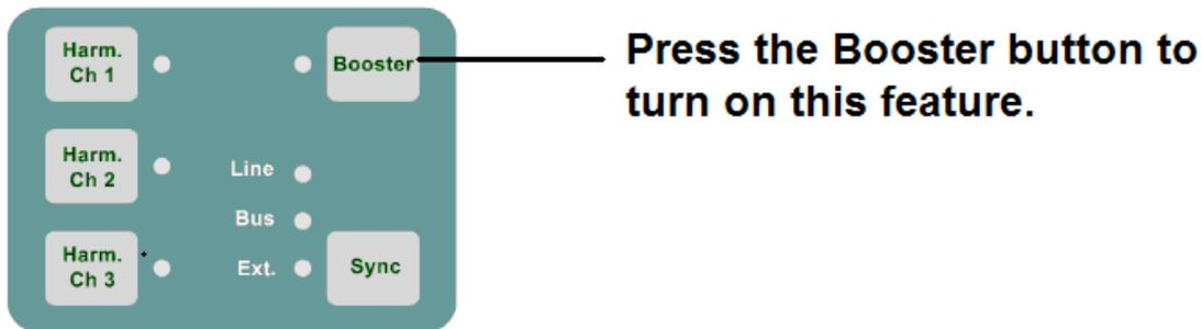
By turning on the booster the voltage available to push the current is doubled. If the booster does not provide enough VA to achieve the desired current refer to paralleling or series the currents.
