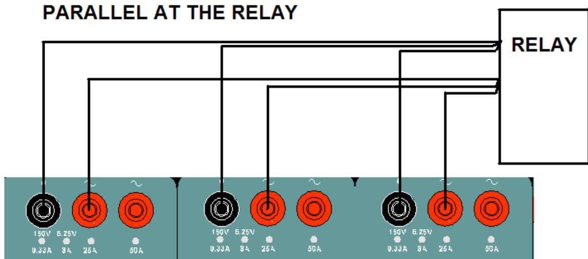
Paralleling at the test set is one of the most common mistakes made. By paralleling at the test set three times the current is passed through one set of test leads instead of sharing that load across three sets of leads.
