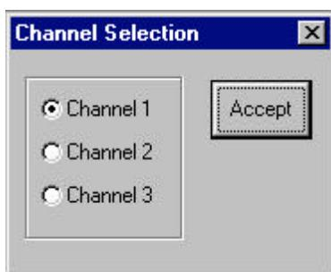
In the case you are adjusting a unit which has more than 1 output channel, another screen will appear and you must select the channel you wish to adjust.
