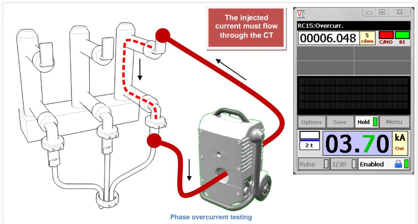
5. Manually set the circuit breaker to CLOSE position if necessary.
