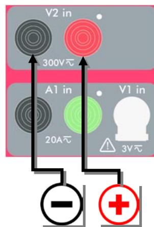
Measuring auxiliary DC voltage
