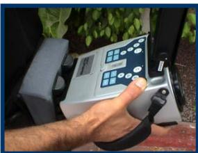
4. Lean the camera against the front pad. Use the grooves to adjust the viewing angle of the camera.
