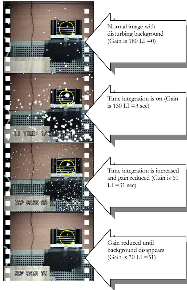
When operating in the LI mode the UV channel of the DayCor® Superb camera turns into a slow response instrument. If the camera moves relative to the UV source the UV image will be smeared. When recording while operating in the LI mode, the camera should preferably be used from a tripod, or the operator should be able to hold the camera without moving it
