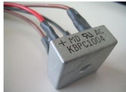
If you are analysing a simple *trip* or *close* operation or if only one of the actuation coils is AC-powered, you will only need to connect one rectifier bridge to the appropriate coil control connections in the PME-500-TR.
